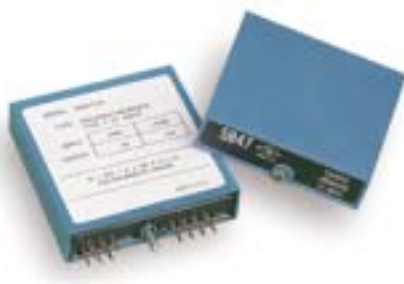
5B modules selected from a choice of types are placed into the WBK15 module
